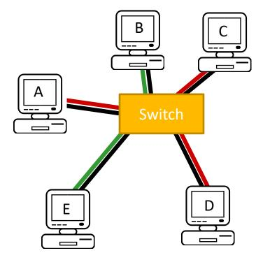
A transmits to D D replies to A E transmits to B, and A to C
